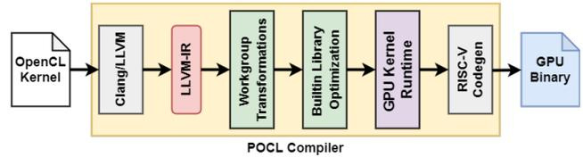
Figure 11: Vortex binary generation steps for OpenCL applications.
