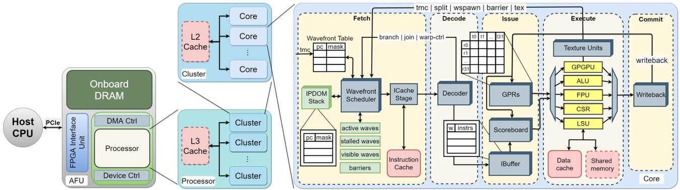
Figure 4: Vortex microarchitecture.
