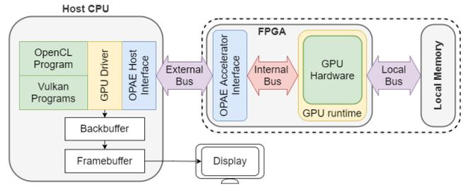
Figure 9: Vortex driver stack and frame buffer connection.
