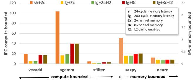
Figure 21: The effect of memory scaling on performance.
