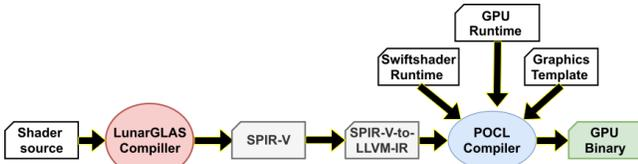
Figure 12: Shader compilation pipeline.
